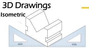
An isometric drawing is a pictorial representation of an object in which all three dimensions are drawn at full scale. It is drawing with all horizontal lines at 30° using the 60/30 set square or using an isometric grid
