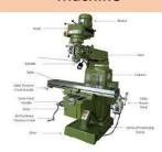
The vertical milling machine is a precision tool used for shaping and fabrication by the removal of stock typically from metallic work pieces
